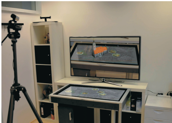
Figure 1. An example application of augmented reality running on the MARS: Bratislava sights are mixed with the interactive map of the old town.
