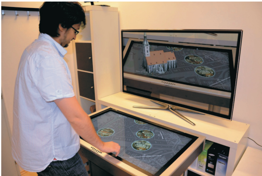
Figure 6: MARS set-up with an interactive map of Bratislava augmented by 3D models of historical sights.
